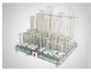
38 nos. of cylinder. To simultaneously wash mearsure cylinder 16 nos. of 5~25ml, 12 nos. of 50~250ml, 6 nos. of 500ml and 4 nos. of 1000~2000ml
